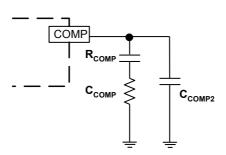
C<sub>COMP2</sub> is needed only for high ESR output capacitor Figure 2. Stability Compensation
