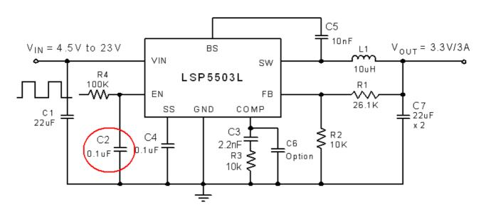
LSP5503L application circuit, 3.3V/3A output with EN function Note: C2 is required for separate EN signal.
