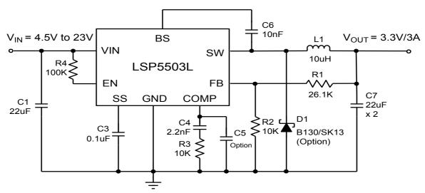
LSP5503L application circuit, 3.3V/3A output.
