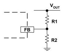
Figure 1. Output Voltage Setting
