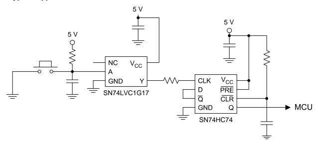
Figure 4. Device Power Button Circuit
