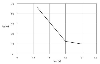
Figure 5. Typical Propagation Delay - CLR to Q
