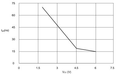
Figure 1. Typical Propagation Delay - CLK to Q
