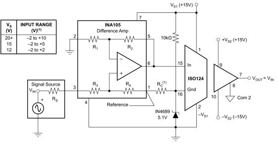
NOTE: Because the amplifier is unity gain, the input range is also the output range. The output can go to -2 V because the output section of the ISO amp operates from dual supplies.
