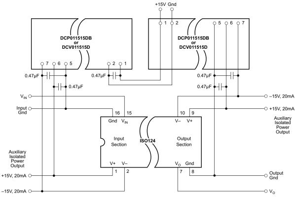
Figure 23. Powered ISO Amplifier With Three-Port Isolation Schematic
