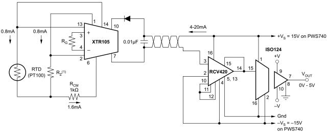
Figure 20. Isolated 4- to 20-mA Instrument Loop (RTD Shown)
