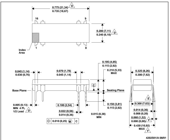
A. All linear dimensions are in inches (millimeters).
