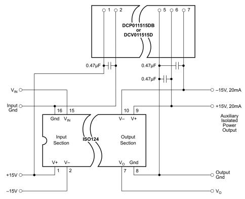
Figure 22. Input-Side Powered ISO Amplifier Schematic
