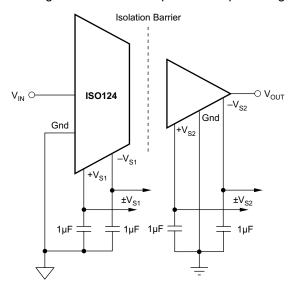
Figure 24. Basic Signal and Power Connections
