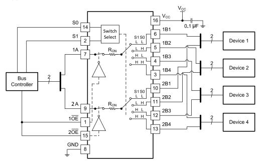
Figure 3. Typical Application of the SN74CBTLV3253
