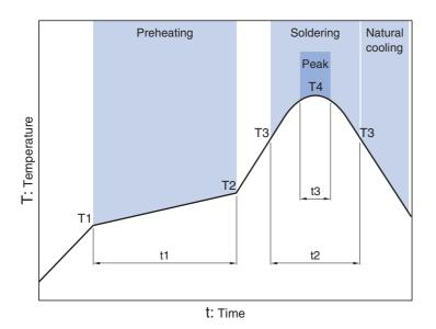
Preheating Soldering Peak Temp. Temp. Time Time Temp. Time **T1** T2 t1 ТЗ t2 Т4 t3 150°C 180°C 60 to 120s 230°C 30 to 50s 250 to 260°C 10s max.
