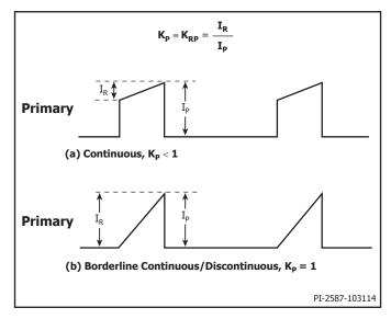
Figure 19. Continuous Mode Current Waveform,  $K_{p} \leq 1$ .
