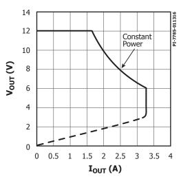
Figure 2 Output Characteristics.
