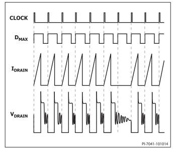
Figure 9. Operation at Near Maximum Loading.
