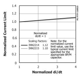
Figure 22. Standard Current Limit Vs. di/dt.
