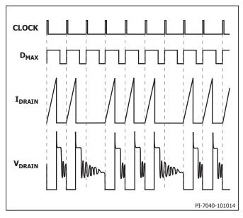
Figure 10. Operation at Moderately Heavy Loading.
