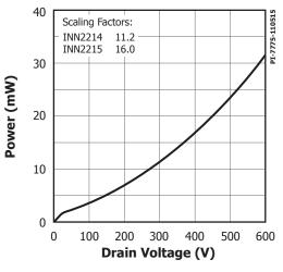
Figure 25. Drain Capacitance Power.
