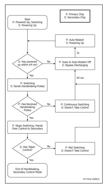
Figure 7. Primary –Secondary Handshake Flowchart.
