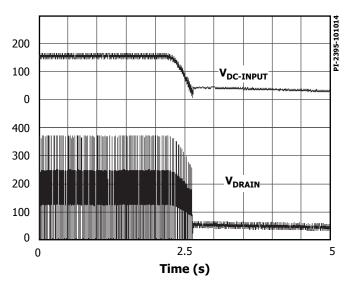
Figure 14. Normal Power-Down Timing.
