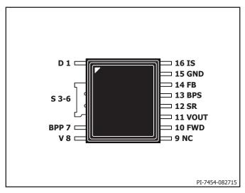
Figure 6. Pin Configuration.
