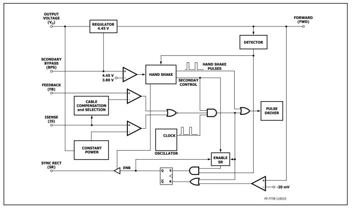
Figure 5. Secondary-Side Controller Block Diagram.
