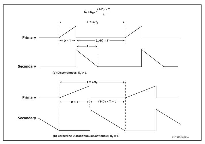
Figure 20. Discontinuous Mode Current Waveform,  $K_p \ge 1$ .
