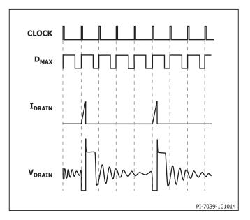
Figure 12. Operation at Very Light Load.
