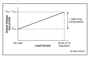
Figure 8. Cable Drop Compensation Characteristics.
