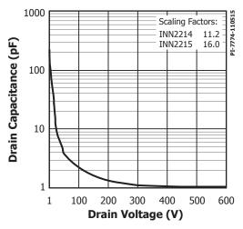
Figure 24. C<sub>oss</sub> vs. Drain Voltage.
