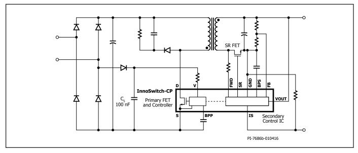
Figure 17. Fast AC Reset Configuration.
