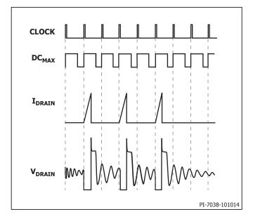
Figure 11. Operation at Medium Loading.
