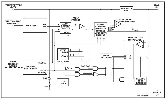
Figure 4. Primary-Side Controller Block Diagram.
