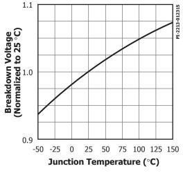
Figure 21. Breakdown vs. Temperature.
