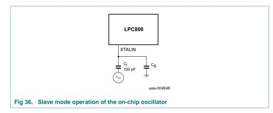
In slave mode the input clock signal should be coupled by means of a capacitor of 100 pF (Figure 36), with an amplitude between 200 mV (RMS) and 1000 mV (RMS). This corresponds to a square wave signal with a signal swing of between 280 mV and 1.4 V. The XTALOUT pin in this configuration can be left unconnected.
