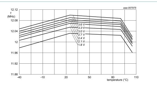
Conditions: Frequency values are typical values. 12 MHz  $\pm$  1.5 % accuracy is guaranteed for 2.7 V  $\leq$  V<sub>DD</sub>  $\leq$  3.6 V and T<sub>amb</sub> = -40 °C to +105 °C. Variations between parts may cause the IRC to fall outside the 12 MHz  $\pm$  1.5 % accuracy specification for voltages below 2.7 V.
