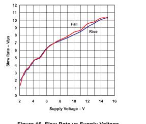
Figure 16. Slew Rate vs Supply Voltage
