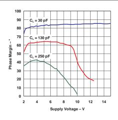
Figure 10. Phase Margin vs Supply Voltage
