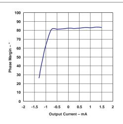
Figure 9. Phase Margin vs Output Current
