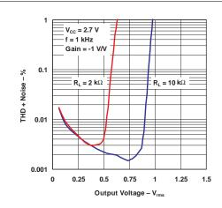
Figure 4. Total Harmonic Distortion + Noise vs Output Voltage
