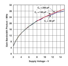
Figure 8. Gain Bandwidth Product vs Supply Voltage
