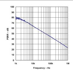
Figure 13. Power-Supply Ripple Rejection vs Frequency
