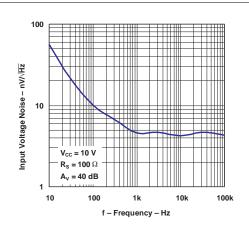
Figure 6. Input Voltage Noise vs Frequency
