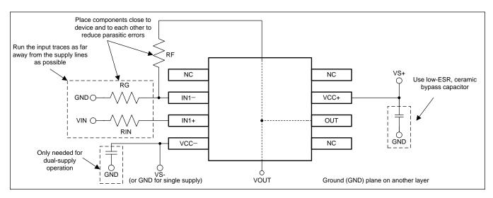
Figure 22. Operational Amplifier Board Layout for Noninverting Configuration
