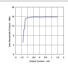
Figure 7. Gain Bandwidth Product vs Output Current
