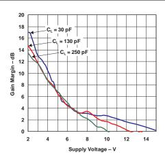
Figure 11. Gain Margin vs Supply Voltage
