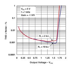
Figure 5. Total Harmonic Distortion + Noise vs Output Voltage
