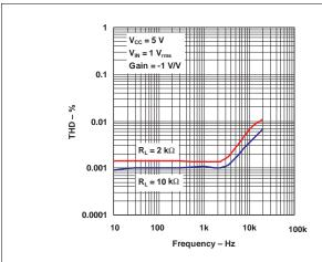
Figure 3. Total Harmonic Distortion vs Frequency
