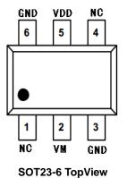
Figure 2. PIN Configuration
