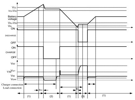
Figure 5-1 Overcharge and Overdischarge Voltage Detection
