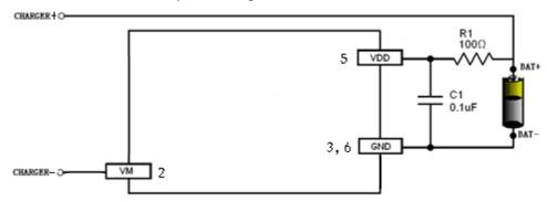
Fig 6 XB5306A in a Typical Battery Protection Circuit
