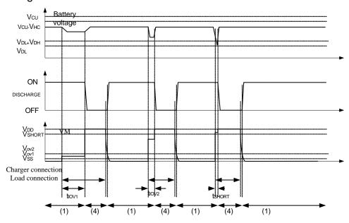
**Figure5-2 Overdischarge Current Detection**
