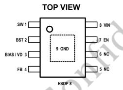
EXPOSED PAD(PIN 9) IS GND, MUST BE SOLDERED TO PCB
