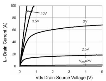
**Figure 1 Output Characteristics**
