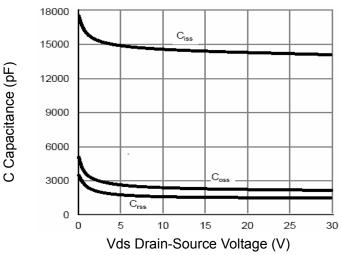
Figure 7 Capacitance vs Vds
