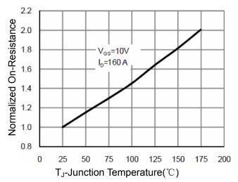
Figure 4 Rdson-JunctionTemperature
