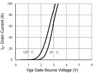
**Figure 2 Transfer Characteristics**
