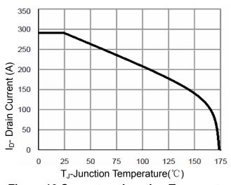
**Figure 10 Current vs Junction Temperature**
