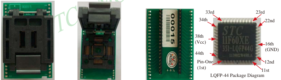
Transition Socket of LQFP44(front) Transition Socket of LQFP44(inside) Transition Socket of LQFP44(back)
