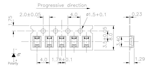
**Note:** Tolerances Unless Dimension  $\pm$  0.1mm, Unit = mm
