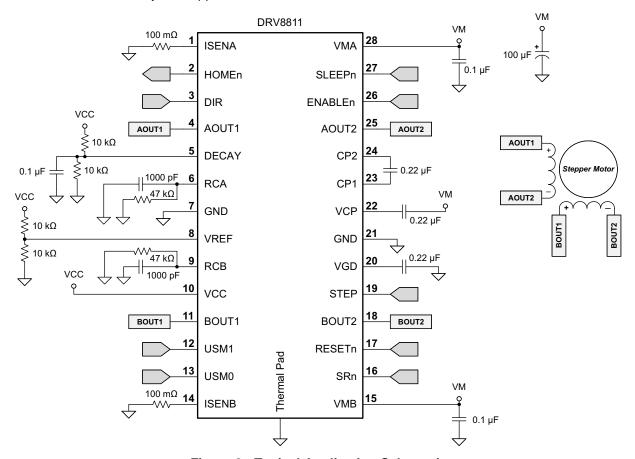
Figure 9. Typical Application Schematic
