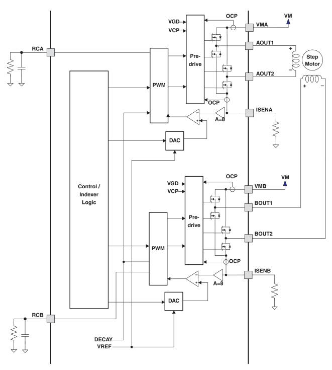
Figure 6. Motor Control Circuitry
