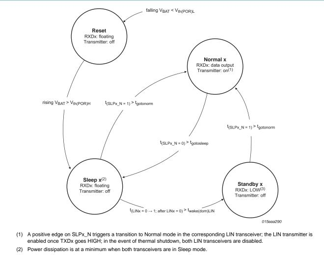
(3) When a transceiver switches to Standby mode in response to a LIN bus wake-up event, the associated RXDx pin (RXD1 or RXD2) will be LOW to indicate which LIN channel was the source of the wake-up request.
