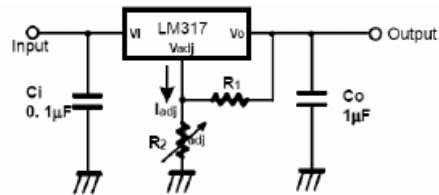
$$V_o = 1.25V \left(1 + \frac{R_2}{R_1}\right) + I_{adj} R_2$$
