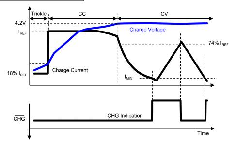
Figure 3. Typical Charge Profile
