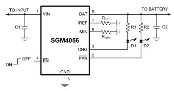
Figure 1. Typical Application Circuit Interfacing to Indication LEDs
