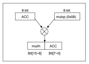
Fig. 14: Block diagram of hardware multiplier
