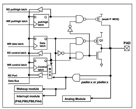
Fig.11: Hardware diagram of IO buffer
