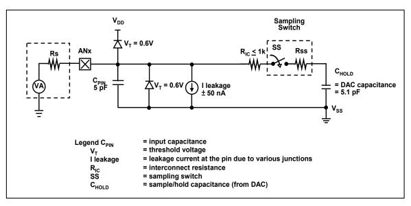
Fig.13: Analog Input Model
