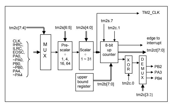
Fig.5: Timer2 hardware diagram
