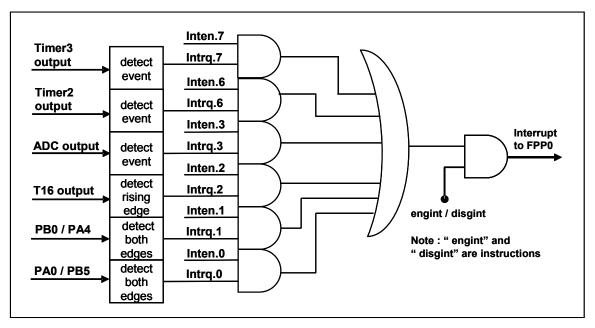
Fig.8: Hardware diagram of interrupt controller
