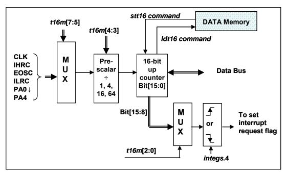
Fig.4: Hardware diagram of Timer16
