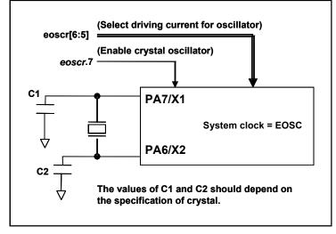
Fig.2: Connection of crystal oscillator
