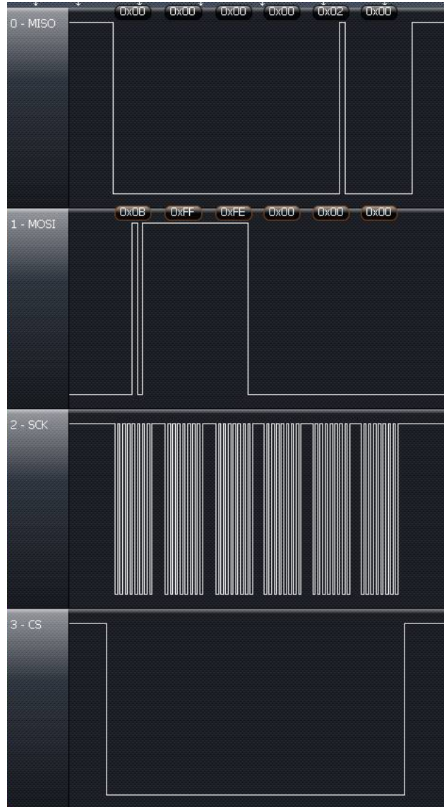
图 5-9. SPI Access Example: Read of the Control Register at Address 0xFFFE, Responds With 0x00, 0x02 (RF Enable = 1)
