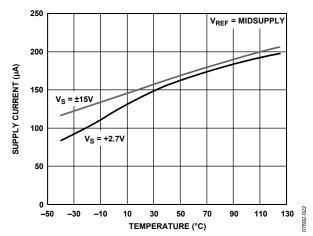
Figure 22. Supply Current vs. Temperature
