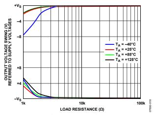
Figure 18. Output Voltage Swing vs.  $R_L$  and Temperature,  $V_S = \pm 15~V$
