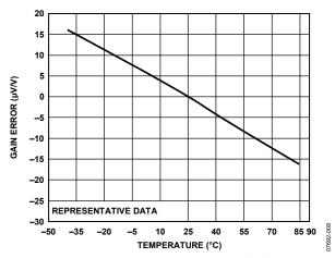
Figure 9. Gain Error vs. Temperature, Normalized at 25°C
