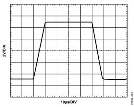
Figure 28. Large-Signal Step Response
