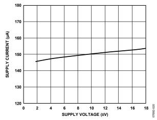
Figure 20. Supply Current vs. Dual Supply Voltage,  $V_{IN} = 0 V$
