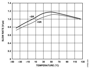
Figure 24. Slew Rate vs. Temperature,  $V_{IN} = 20 \text{ V p-p}$ , 1 kHz
