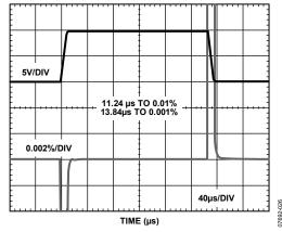
Figure 26. Large-Signal Pulse Response and Settling Time, 10 V Step,  $V_S = \pm 15 \text{ V}$
