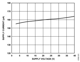
Figure 21. Supply Current vs. Single-Supply Voltage,  $V_{IN} = 0 V$ ,  $V_{REF} = 0 V$
