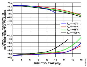
Figure 17. Output Voltage Swing vs. Supply Voltage and Temperature,  $R_L = 2 \, k \Omega$
