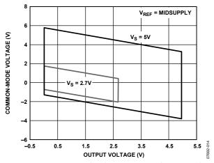
Figure 14. Input Common-Mode Voltage vs. Output Voltage, 5 V and 2.7 V Supplies,  $V_{\it REF} = Midsupply$
