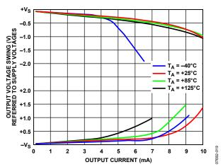
Figure 19. Output Voltage Swing vs.  $I_{OUT}$  and Temperature,  $V_S = \pm 15V$
