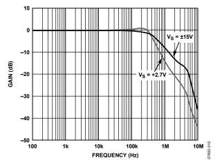
Figure 10. Gain vs. Frequency,  $V_S = \pm 15 V$ , +2.7 V
