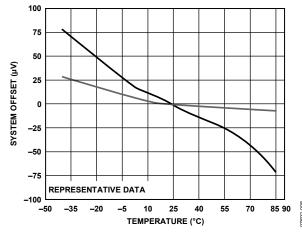
Figure 8. System Offset vs. Temperature, Normalized at 25°C
