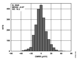
Figure 6. Distribution of Typical Common-Mode Rejection
