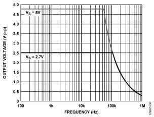
Figure 30. Maximum Output Voltage vs. Frequency,  $V_S = 5 V$ , 2.7 V
