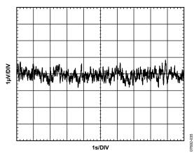
Figure 34. 0.1 Hz to 10 Hz Voltage Noise
