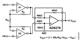
Figure 44. Low Power Precision Instrumentation Amplifier
