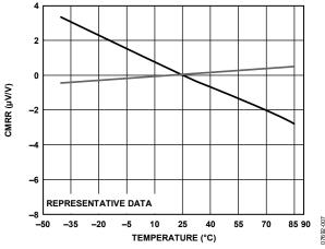
Figure 7. CMRR vs. Temperature, Normalized at 25°C
