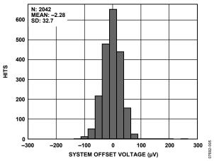
Figure 5. Distribution of Typical System Offset Voltage
