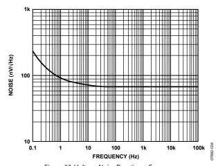
Figure 33. Voltage Noise Density vs. Frequency
