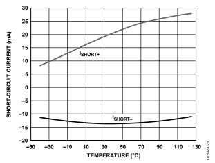
Figure 23. Short-Circuit Current vs. Temperature
