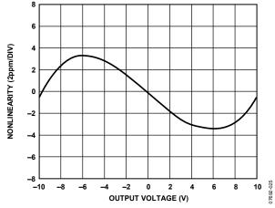
Figure 25. Gain Nonlinearity,  $V_S = \pm 15 \text{ V}$ ,  $R_L \ge 2 \text{ k}\Omega$
