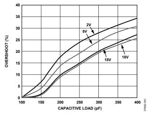
Figure 32. Small-Signal Overshoot vs. Capacitive Load,  $R_L \ge 2 k\Omega$
