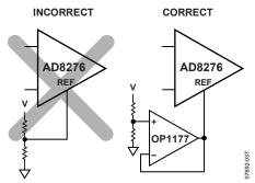
Figure 37. Driving the Reference Pin
