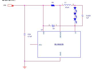
A value of 1uF will reduce the supply ripple current by a factor three (approx.). Proportionally lower ripple can be achieved with higher capacitor values. Note that the capacitor will not affect operating frequency or efficiency, but it will increase start-up delay and reduce the frequency of
