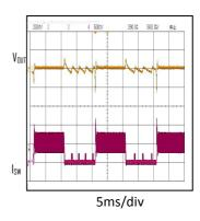
Load Transient Response VIN=12V,VOUT=5V,IOUT=0 to 0.5A Short-Circuit Response VIN=24V,VOUT=5V,IOUT=0A to Short-Circuit Recovery
