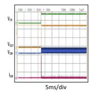
Start-up Waveform with EN=VIN VIN=12V,VOUT=5V,IOUT=0A
