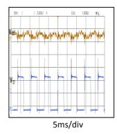
Load Transient Response VIN=12V,VOUT=3.3V,IOUT=0 to 0.5A
