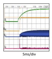
Shutdown Waveform with EN VIN=30V,VOUT=5V,IOUT=0.5A
