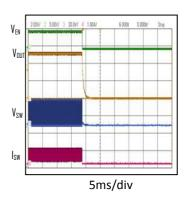
Switching Waveform VIN=12V,VOUT=5V,IOUT=0.1A
