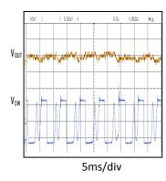
Switching Waveform VIN=12V,VOUT=5V,IOUT=0.3A
