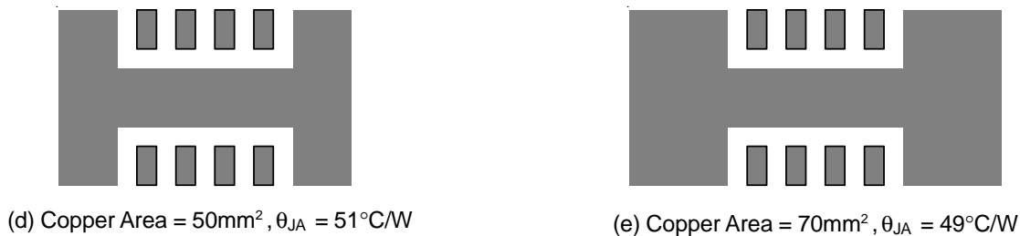
Figure 6. Thermal Resistance vs. Copper Area Layout Design
