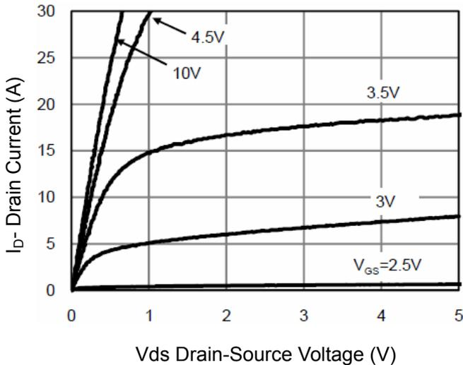
Figure 3 Output Characteristics
