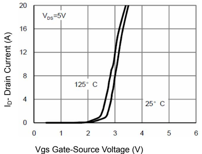
Figure 4 Transfer Characteristics
