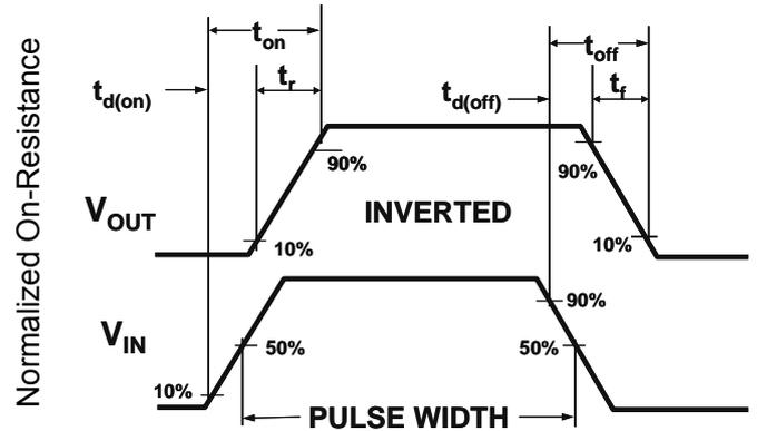
Figure 2: Switching Waveforms
