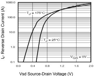
Figure 6 Source- Drain Diode Forward
