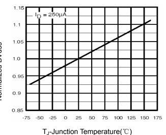
Figure 10 BV<sub>DSS</sub> vs Junction Temperature
