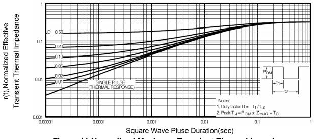
Figure 11 Normalized Maximum Transient Thermal Impedance
