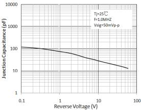
Figure 4. Typical Junction Capacitance
