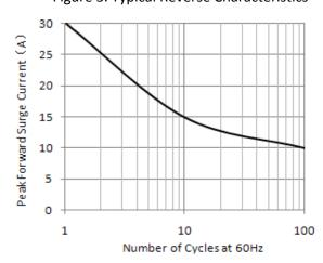
Figure 5.Maximum Non-Repetitive Peak Forward Surge Current
