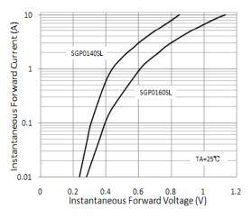
Figure 2. Typical Instantaneous Forward Characteristics
