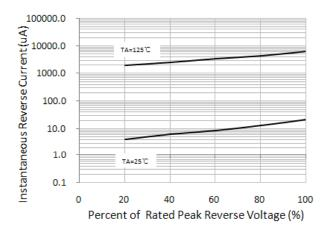
Figure 3. Typical Reverse Characteristics
