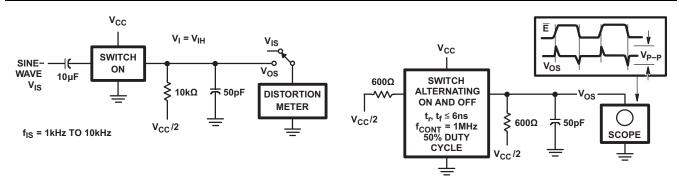
Figure 12. ¼Sine-Wave Distortion Test Circuit
