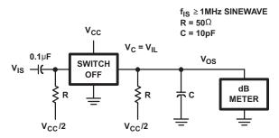
Figure 14. Switch OFF Signal Feedthrough
