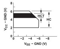
Figure 2. Recommended Operating Area as a Function of (V<sub>EE</sub> – GND)
