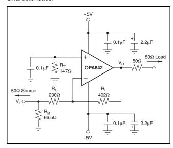
Figure 38. Inverting G = -2 Specifications and Test Circuit
