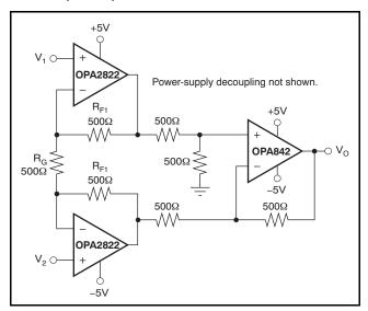
Figure 40. Wideband Three-Op Amp Differencing Amplifier
