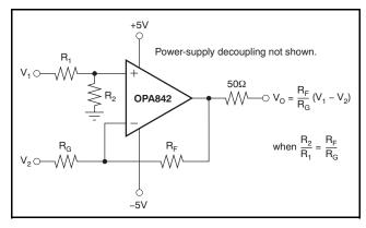
Figure 39. High-Speed, Single Differential Amplifier
