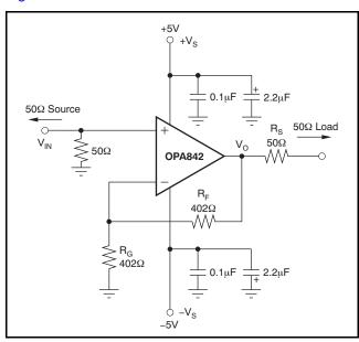
Figure 37. Gain of +2, High-Frequency Application and Characterization Circuit
