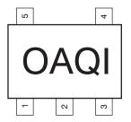
Pin Orientation/Package Marking
