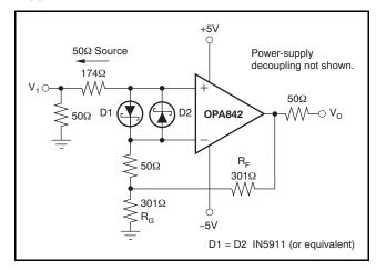
Figure 45. Gain of +2 with Input Protection
