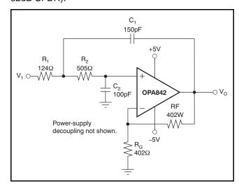
Figure 42. 5MHz Butterworth Low-Pass Active Filter
