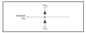
Figure 44. Internal ESD Protection
