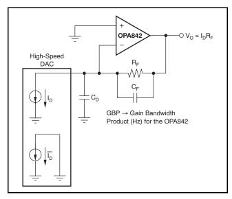
Figure 41. Wideband, Low-Distortion DAC Transimpedance Amplifier
