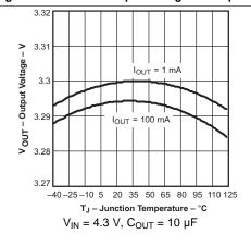
Figure 4. TPS79133 Output Voltage vs **Junction Temperature**
