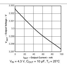
Figure 2. TPS79133 Output Voltage vs Output Current
