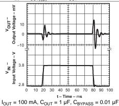
Figure 25. TPS79118 Line Transient Response
