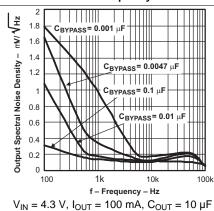
Figure 11. TPS79133 Output Spectral Noise Density vs Frequency
