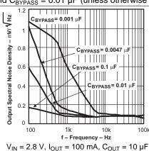
Figure 8. TPS79118 Output Spectral Noise Density vs Frequency
