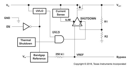
Figure 33. Functional Block Diagram: Fixed Version
