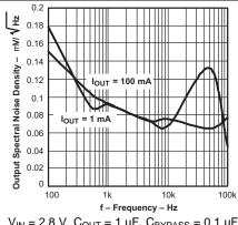
$V_{IN}$  = 2.8 V,  $C_{OUT}$  = 1  $\mu F,~C_{BYPASS}$  = 0.1  $\mu F$
