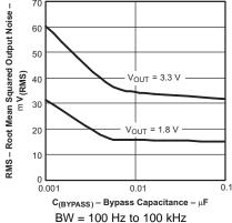
Figure 12. Root Mean Squared Output Noise vs **Bypass Capacitance**
