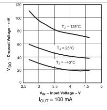
Figure 16. TPS79101 Dropout Voltage vs Input Voltage
