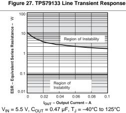
Figure 29. TPS79118 Typical Regions of Stability Equivalent Series Resistance (ESR) vs Output Current
