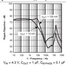
Figure 23. TPS79133 Ripple Rejection vs Frequency
