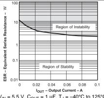
$V_{IN}$  = 5.5 V,  $C_{OUT}$  = 1  $\mu$ F,  $T_J$  = -40°C to 125°C
