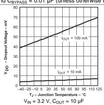
Figure 14. TPS79133 Dropout Voltage vs Junction Temperature
