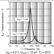
Figure 13. TPS79133 Output Impedance vs Frequency
