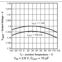
Figure 3. TPS79118 Output Voltage vs **Junction Temperature**
