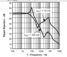
$V_{IN} = 2.8 \text{ V}, C_{OUT} = 1 \mu\text{F}, C_{BYPASS} = 0.1 \mu\text{F}$
