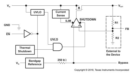
Figure 32. Functional Block Diagram: Adjustable Version
