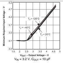
Figure 17. Minimum Required Input Voltage vs **Output Voltage**
