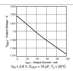
Figure 1. TPS79118 Output Voltage vs Output Current
