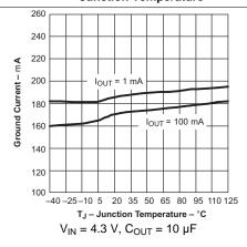
Figure 5. TPS79133 Ground Current vs **Junction Temperature**
