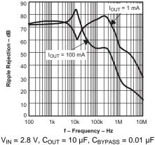
Figure 18. TPS79118 Ripple Rejection vs Frequency
