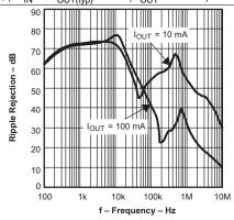
$V_{IN} = 2.8 \text{ V}, C_{OUT} = 1 \mu\text{F}, C_{BYPASS} = 0.01 \mu\text{F}$
