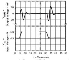
$I_{OUT}$  = 100 mA,  $C_{OUT}$  = 1  $\mu F,~C_{BYPASS}$  = 0.01  $\mu F,$  $dv / dt = 0.4 V / m_s$
