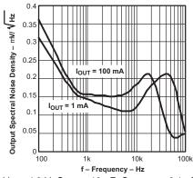
$V_{IN}$  = 4.3 V,  $C_{OUT}$  = 10  $\mu$ F,  $C_{BYPASS}$  = 0.1  $\mu$ F
