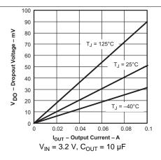
Figure 15. TPS79133 Dropout Voltage vs Output Current
