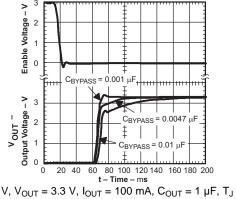
$V_{IN} = 4.3~V,~V_{OUT} = 3.3~V,~I_{OUT} = 100~mA,~C_{OUT} = 1~\mu F,~T_{J} = 25^{\circ}C$
