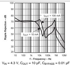
Figure 20. TPS79118 Ripple Rejection vs Frequency
