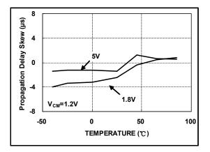
Propagation Delay vs. Temperature
