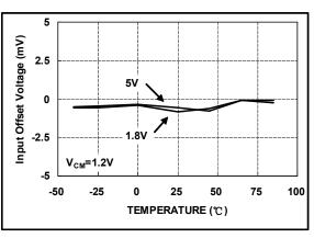
Input Offset Voltage vs. Temperature
