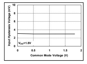
Input Hysteresis Voltage vs. Common Mode Voltage
