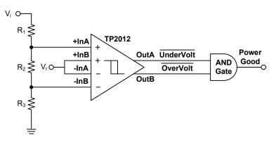
Figure 9. Windowed Comparator
