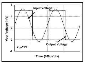
Figure 1. Comparator Response to Input Voltage
