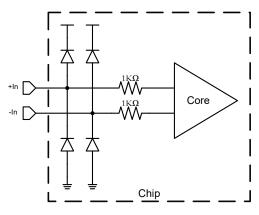
Figure 2. Equivalent Input Structure
