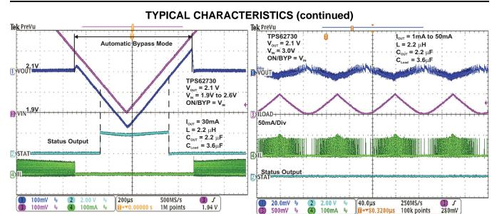
Figure 21. Automatic Bypass Transition with Falling / Rising Input Voltage  $\rm V_{\rm IN}$
