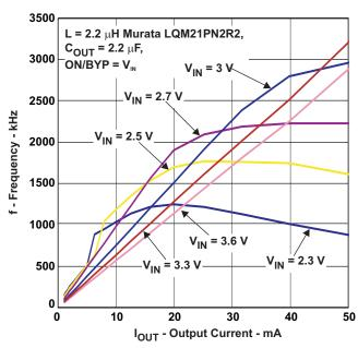
Figure 12. Switching Frequency vs I<sub>OUT</sub> vs V<sub>IN</sub>
