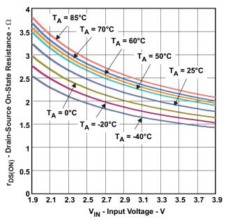
Figure 7. r<sub>DS(ON)</sub> Bypass vs Input Voltage
