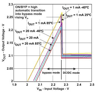
Figure 11. Automatic Transition into Bypass Mode - Rising  $V_{\rm IN}$
