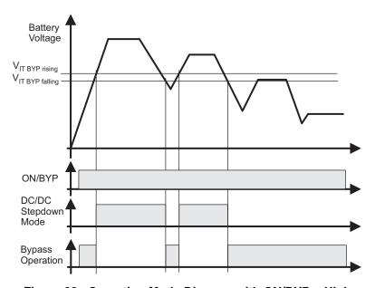
Figure 28. Operation Mode Diagram with ON/BYP = High
