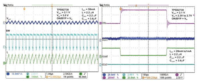
Figure 19. DC/DC Mode Operation I<sub>OUT</sub> = 50mA
