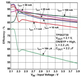
Figure 2. Efficiency vs Input Voltage
