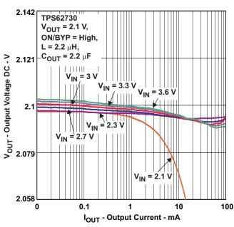
Figure 3. Output Voltage vs Output Current
