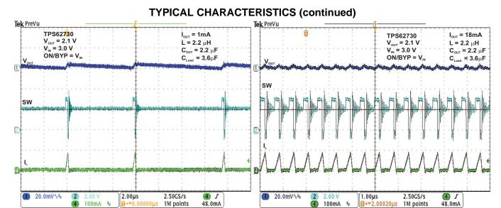
Figure 17. DC/DC Mode Operation I<sub>OUT</sub> = 1mA
