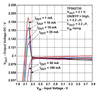
Figure 4. Output Voltage vs Input Voltage
