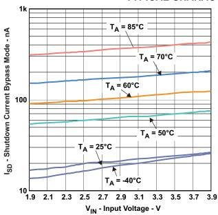
Figure 5. Shutdown Current Bypass Mode vs Input Voltage
