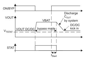
Figure 29. Signal Status Diagram ON/BYP, VOUT, STAT
