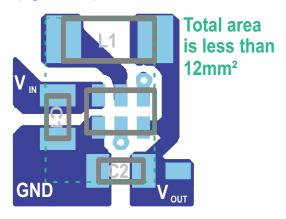
Figure 33. Recommended PCB Layout for TPS62730
