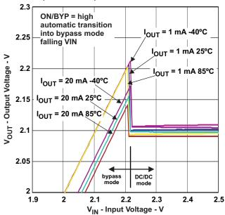
Figure 10. Automatic Transition into Bypass Mode - Falling  $V_{\text{IN}}$
