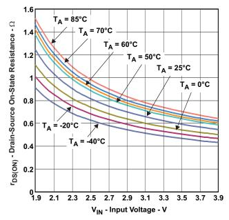
Figure 8.  $r_{DS(ON)}$  PMOS vs Input Voltage
