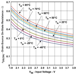
Figure 9. r<sub>DS(ON)</sub> NMOS vs Input Voltage
