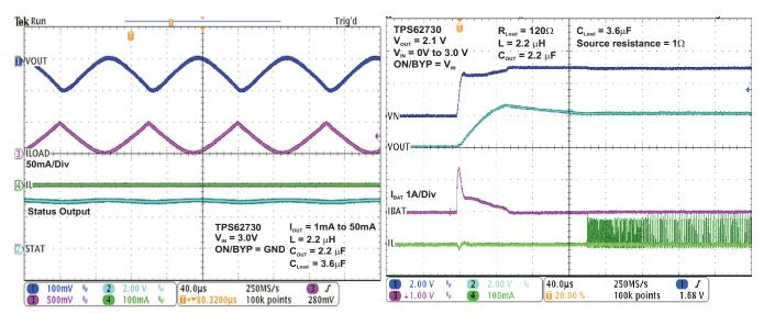
Figure 23. Bypass Mode Operation  $V_{OUT}$  AC Behavior ON/BYP = GND
