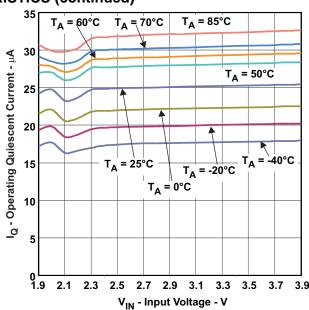
Figure 6. Operating Quiescent Current vs Input Voltage
