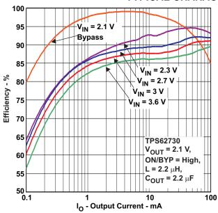
Figure 1. Efficiency vs Output Current
