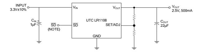
Notes: 1.  $\overline{\text{SD}}$  pins must be pulled high through a 10k $\Omega$  pull-up resistor.
