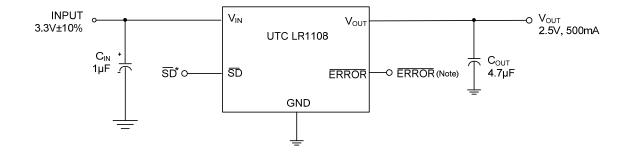
Note:  $\overline{SD}$  and  $\overline{ERROR}$  pins must be pulled high through a 10k $\Omega$  pull-up resistor. Connect the  $\overline{ERROR}$  pin to ground if this function is not used.
