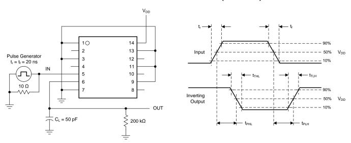
Figure 14. Dynamic Electrical Characteristics Test Circuit and Waveform
