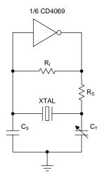
Figure 15. Typical Crystal Oscillator Circuit
