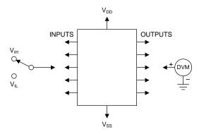
Figure 12. Noise Immunity Test Circuit
