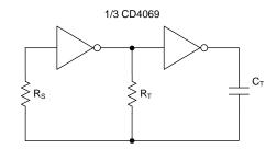
Figure 17. Typical RC Oscillator Circuit
