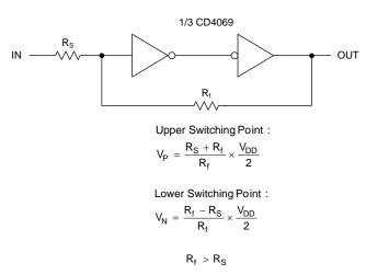
Figure 18. Input Pulse Shaping Circuit
