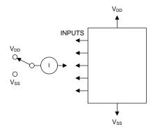
Figure 13. Input Leakage Current Test Circuit
