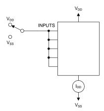
Figure 11. Quiescent Device Current Test Circuit
