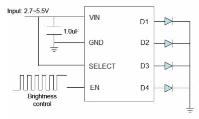
Figure 2: Application Circuit for Co-Cathode Connection.
