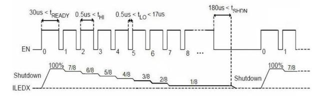
Figure 4: Brightness Control by Pulse Dimming
