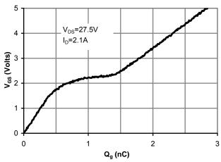
Figure 7: Gate-Charge Characteristics
