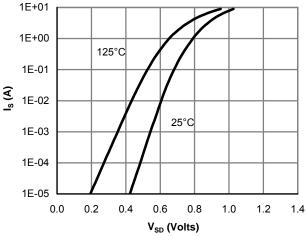
Figure 6: Body-Diode Characteristics
