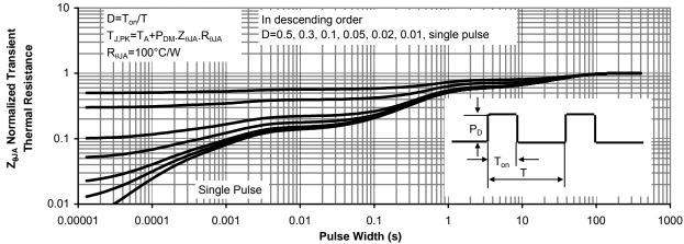
Figure 11: Normalized Maximum Transient Thermal Impedance
