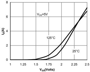
Figure 2: Transfer Characteristics
