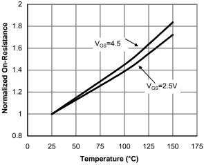
Figure 4: On-Resistance vs. Junction Temperature
