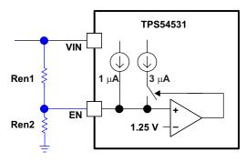
Figure 9. Adjustable Input Undervoltage Lockout
