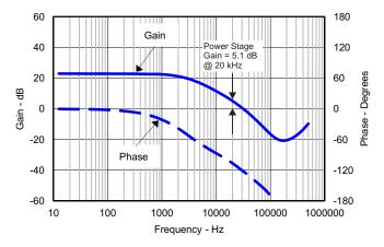
Figure 11. Power Stage Gain and Phase Characteristics
