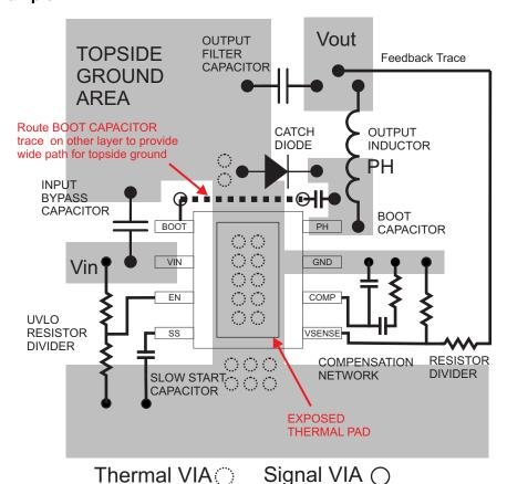
Figure 25. TPS54531DDA Board Layout
