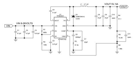
Figure 10. Typical Application Schematic
