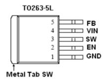
Figure 2. Pin Configuration of XL6006 (Top View)
