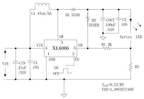
Figure 11. XL6006 System Test Circuit (LED OVP)
