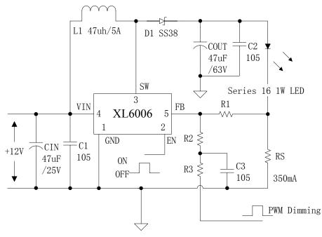
Figure 10. XL6006 System Test Circuit (12V ~16 x 1W LED with Dimming Function)
