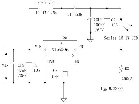
Figure 4. XL6006 Typical Application Circuit
