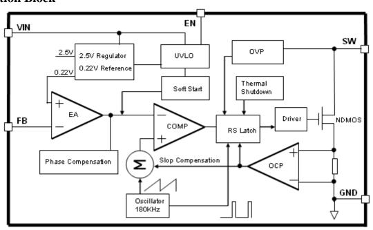
Figure 3. Function Block Diagram of XL6006
