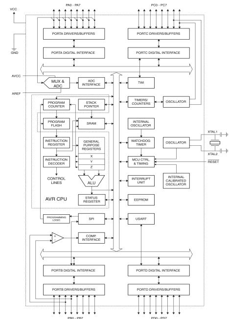
Figure 2-1. Block Diagram
