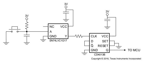
Figure 9. Power Button Circuit
