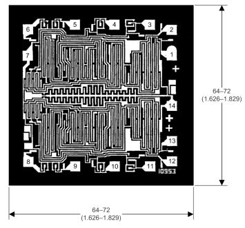
Figure 12. Dimensions and Pad Layout for CD4013B
