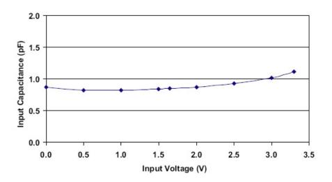
Figure 1. Typical Variation of C<sub>IN</sub> vs. V<sub>IN</sub> (f = 1 MHz, V<sub>P</sub> = 3.3 V, V<sub>N</sub> = 0 V, 0.1  $\mu$ F Chip Capacitor between V<sub>P</sub> and V<sub>N</sub>, 25°C)
