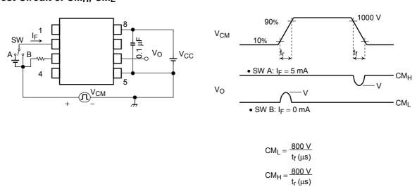
$\mathrm{CM_L}$  (CMH) is the maximum rate of rise (fall) of the common mode voltage that can be sustained with the output voltage in the low (high) state.
