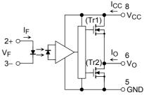
A 0.1  $\mu$ F bypass capacitor must be connected between pin 8 and 5. (See Note 6)
