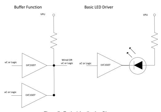
Figure 7. Typical Application Diagram
