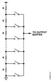
Figure 38. Simplified Resistor String Structure
