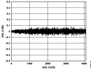
Figure 13. ADC DNL,  $V_{DD} = 2.7 V$
