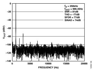
Figure 27. DAC Sine Wave Output, Output Range = 0 V to  $2 \times V_{REF}$ ,
