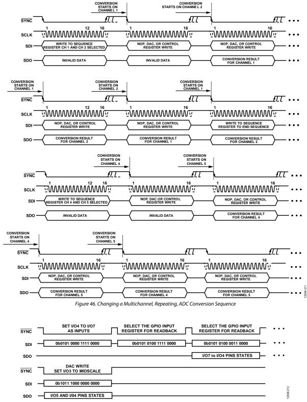
Figure 47. Configuring and Reading General-Purpose Input Pins
