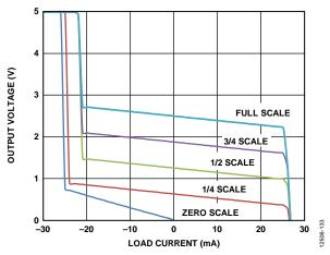
Figure 32. DAC Output Sink and Source Capability, Output Range =  $0 \text{ V to V}_{REF}$
