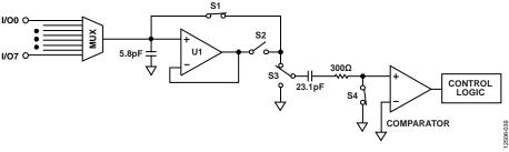
Figure 39. ADC Input Structure
