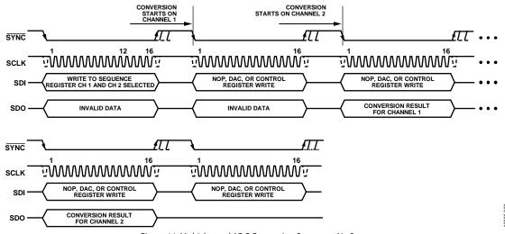
Figure 44. Multichannel ADC Conversion Sequence, No Repeat
