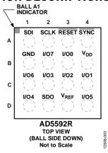
Figure 5. AD5592R 16-Ball WLCSP Pin Configuration
