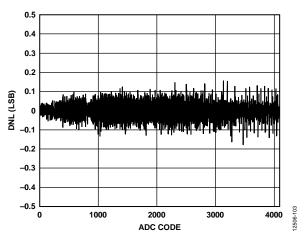
Figure 11. ADC DNL,  $V_{DD} = 5.5 V$
