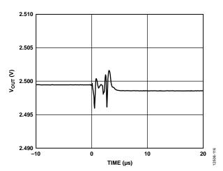
Figure 21. DAC Digital-to-Analog Glitch (Falling)
