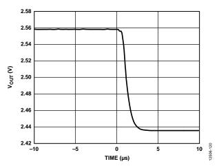
Figure 23. DAC Settling Time (100 Code Change, Falling Edge)
