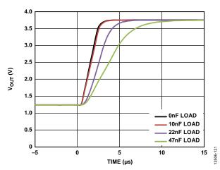
Figure 26. DAC Settling Time for Various Capacitive Loads
