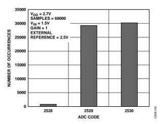
Figure 14. Histogram of ADC Codes,  $V_{DD} = 2.7 \text{ V}$
