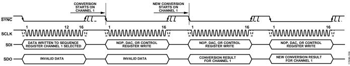
Figure 43. Single-Channel, Repeating, ADC Conversion Sequence
