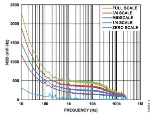
Figure 31. DAC Output Noise Spectral Density (NSD)
