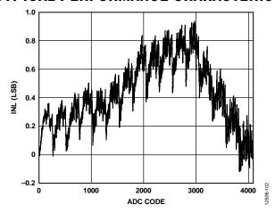
Figure 10. ADC INL,  $V_{DD} = 5.5 V$
