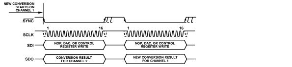
Figure 45. Multichannel, Repeating, ADC Conversion Sequence
