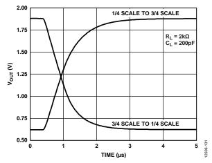
Figure 24. DAC Settling Time, Output Range =  $0 V \text{ to } V_{REF}$
