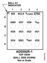
Figure 9. AD5592R-1 16-Ball WLCSP Pin Configuration
