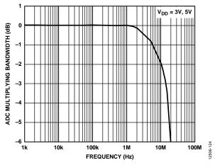
Figure 16. ADC Multiplying Bandwidth
