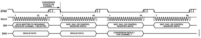
Figure 42. Single-Channel ADC Conversion Sequence, No Repeat
