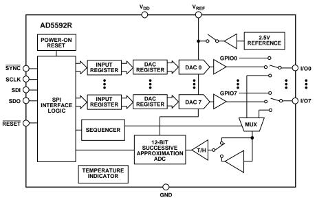
Figure 1. AD5592R Functional Block Diagram
