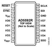
Figure 6. AD5592R 16-Lead TSSOP Pin Configuration
