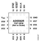
Figure 7. AD5592R 16-Lead LFCSP Pin Configuration
