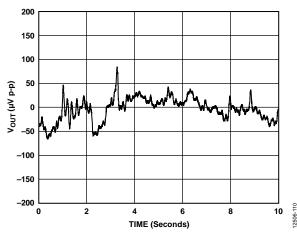
Figure 30. DAC 1/f Noise with Internal Reference
