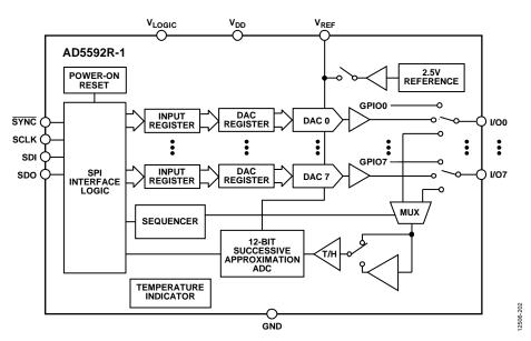
Figure 2. AD5592R-1 Functional Block Diagram
