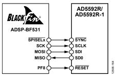
Figure 48. ADSP-BF531 SPI Interface
