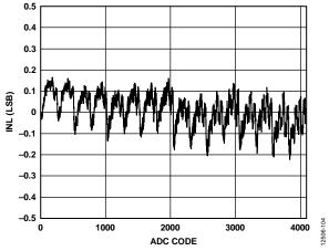
Figure 12. ADC INL,  $V_{DD} = 2.7 V$
