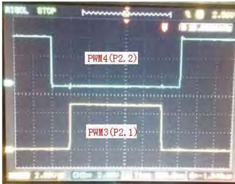
图3: 某个时刻PWM波形, 2V/DIV, 500nS/DIV
