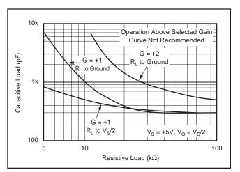
FIGURE 5. Stability-Capacitive Load vs Resistive Load.
