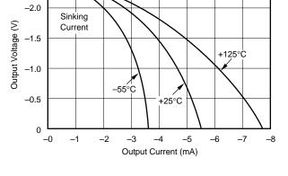
OUTPUT VOLTAGE SWING vs OUTPUT CURRENT
