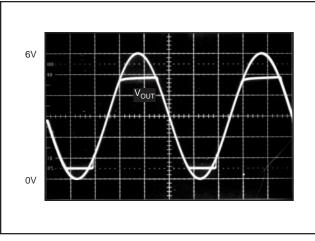
FIGURE 1. No Phase Inversion with Inputs Greater than the Power-Supply Voltage.
