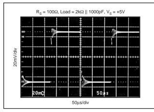
FIGURE 4. Small-Signal Step Response Using Series Resistor to Improve Capacitive Load Drive.
