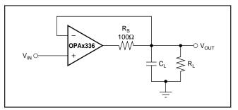
FIGURE 3. Series Resistor in Unity-Gain Configuration Improves Capacitive Load Drive.
