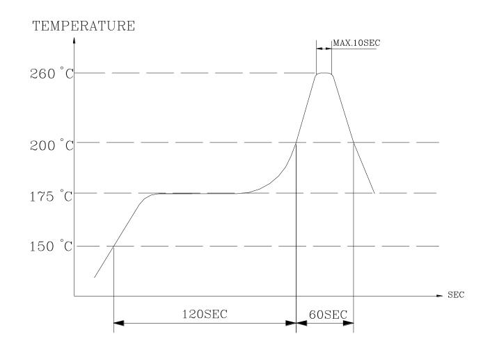
Heat resistant line (Used when heat resistant reliablity test is performed) (2)Manual soldering
