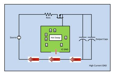
Figure 47. LM5069 Quiet IC Ground Layout
