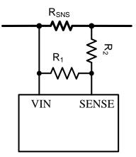
Figure 29. SENSE Resistor Divider
