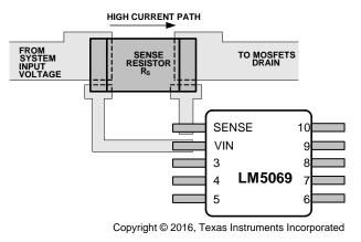
Figure 46. Sense Resistor Connections
