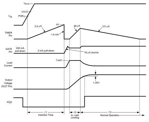
Figure 22. Power-Up Sequence (Current Limit Only)
