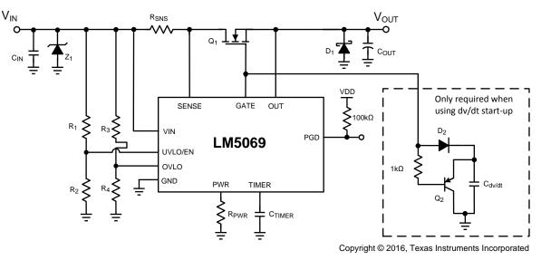
Figure 27. Typical Application Schematic
