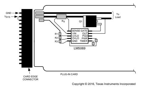
Figure 45. Recommended Board Connector Design
