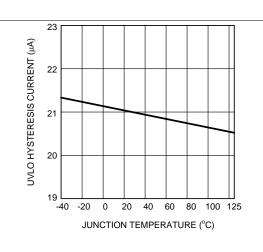
Figure 9. UVLO Hysteresis Current vs Temperature
