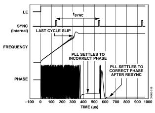
Figure 24. Phase Resync Example
