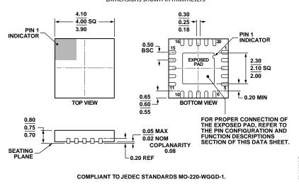
Figure 26. 20-Lead Lead Frame Chip Scale Package [LFCSP\_WQ] 4 mm × 4 mm Body, Very Very Thin Quad (CP-20-6) Dimensions shown in millimeters
