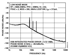
Figure 6. Phase Noise and Spurs, Low Noise Mode
