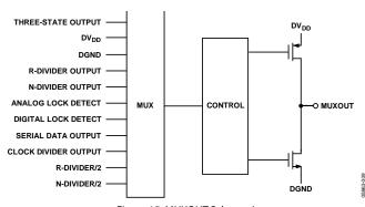
Figure 15. MUXOUT Schematic
