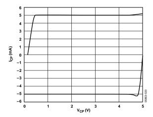
Figure 10. Charge-Pump Output Characteristics
