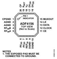
Figure 4. LFCSP Pin Configuration
