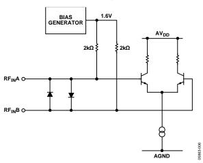
Figure 12. RF Input Stage
