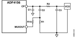
Figure 23. Topology 2—Fast-Lock Loop Filter Topology
