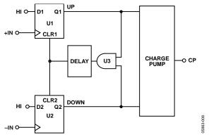
Figure 14. PFD Simplified Schematic
