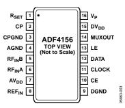
Figure 3. TSSOP Pin Configuration
