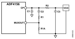
Figure 22. Topology 1—Fast-Lock Loop Filter Topology
