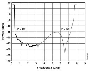
Figure 5. RF Input Sensitivity
