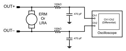
Figure 8. Alternate Test Setup
