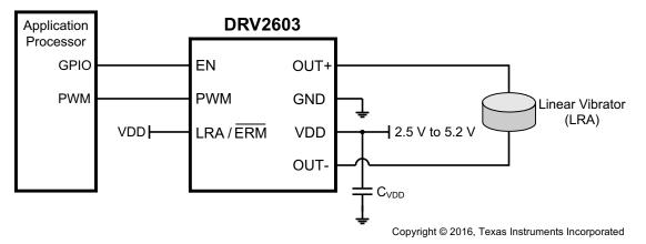
Figure 13. System Diagram for LRA
