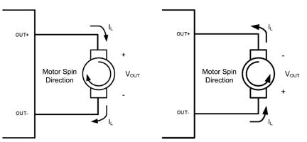
Figure 10. Reversal of Motor Direction
