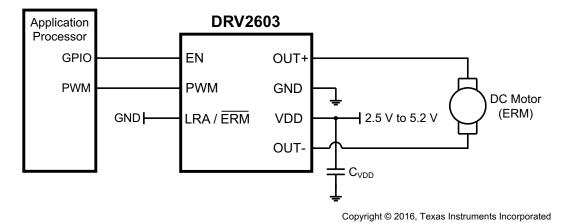
Figure 14. System Diagram for ERM
