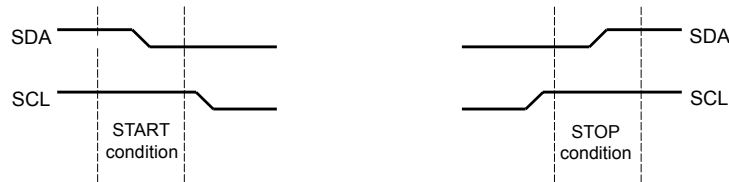
Figure 18-3. START and STOP Conditions
